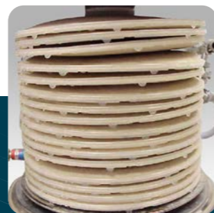
Figure 4: Cell deformities after heat treatment
