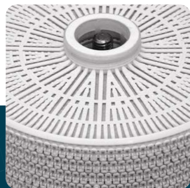
Figure 9: No damage to the SUPRAdisc II modules
