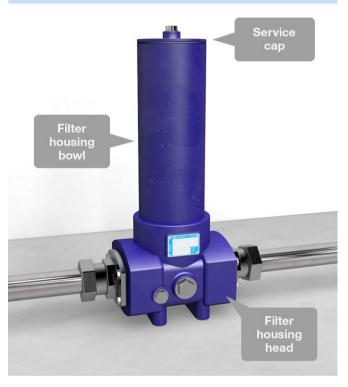
The traditional downward facing filter bowl is now replaced with an upward facing tube with an integral service cap. Once depressurized, just a small volume of service fluid needs to be drained. The easy to access filter cap, weighing just a few pounds (kilo's) on even the largest of filters and significantly less than the previous bowl design, is unscrewed to access and replace the filter element.
