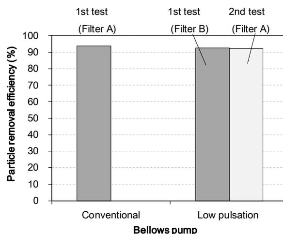
Fig. 5. Results of particle challenge tests in 90 °C sulfuric acid. Two 5-nm-rated PTFE filters (Filters A&B) were evaluated in the recirculation system with each different bellows pump. The flow rate was 16 L/min. Filter A firstly used for the conventional pump was also tested using the low pulsation pump.
