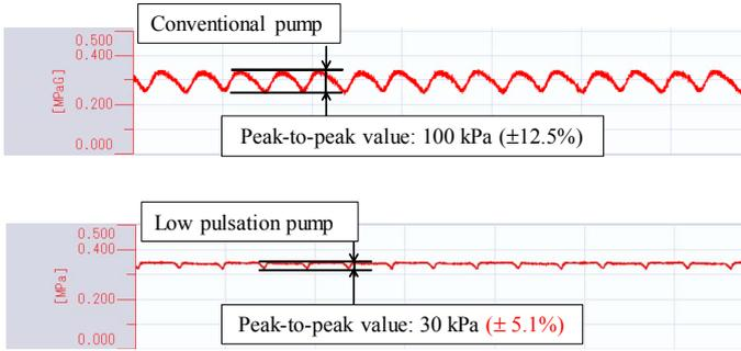
Fig. 2. An example of pulsation of a conventional and a newly developed pump in water. The pressure for discharge is around 0.3 MPa for each data.
