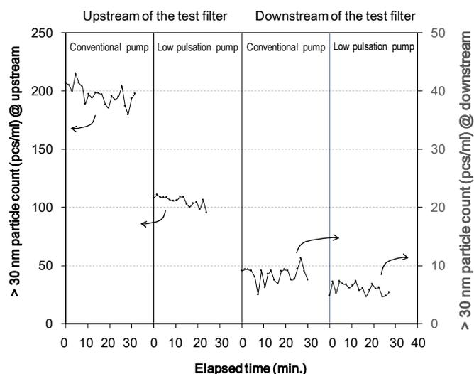
Fig. 4. Particle counts downstream (i.e. upstream and downstream of test filter) of each pump in 90 °C sulfuric acid. Flow rate was 16 L/min.
