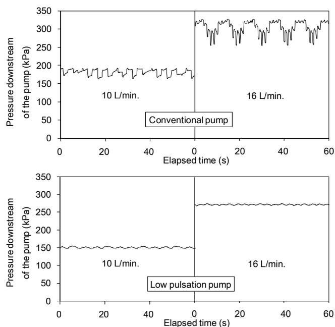
Fig. 3. Pressure fluctuation with time at the downstream of each bellows pump (upstream of each test filter) in 90 °C sulfuric acid.
