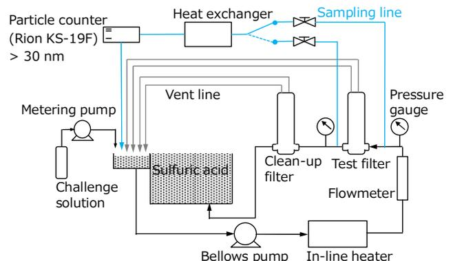
Fig. 1. Schematic of chemical recirculation system used for evaluation of filters and bellows pumps in 90 °C sulfuric acid.
