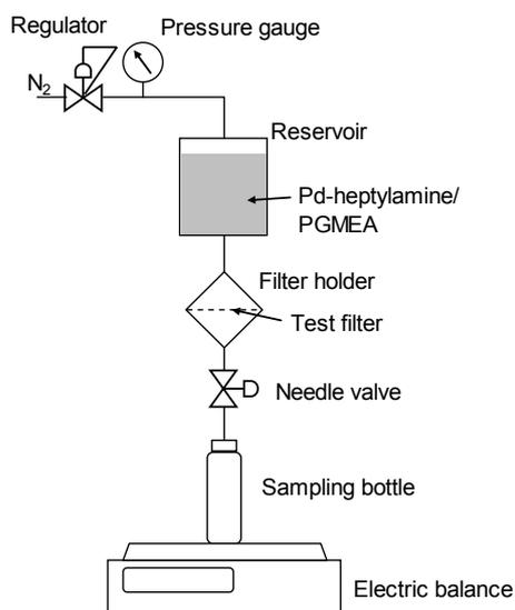
Figure 6 Pressurized flow filtration test stand.
