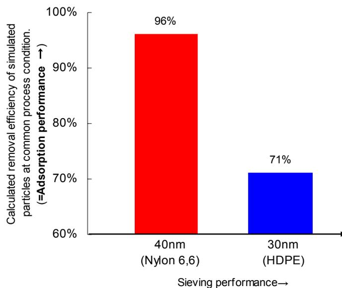
Figure 8. Adsorption and sieving performances of filter products. Adsorption performance is based on adsorption parameters determined by simulation particle filtration testing. Sieving performance is expressed as the established removal rating.
