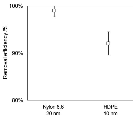
Figure 3 Microbridge removal efficiency\* in 193 nm lithography<sup>[5]</sup> (L/S 90 nm hp). Resist solvent: PGMEA \*: Removal efficiency = 1 - (microbridge defect density on wafer with test filter)/(microbridge defect density on wafer with dummy capsule). Typical flow rate of the photoresist point of use filtration is 0.5 ml/sec.
