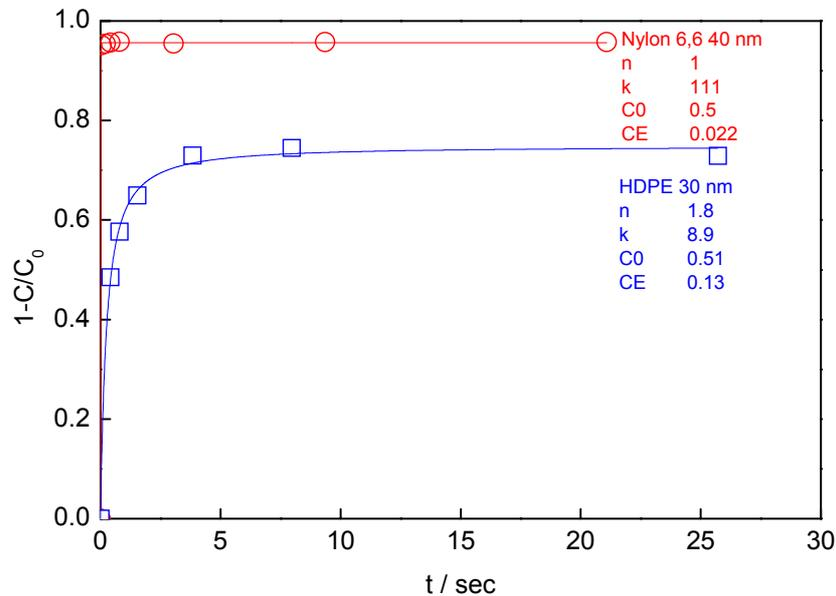
Figure 7. Contact time dependence of simulation particle removal efficiency ( $1 - \frac{C}{C_0}$ ) for Nylon 6,6 40 nm and HDPE 30 nm filters. Continuous lines are fitted adsorption rate equations. Simulation particle is Pd-Heptylamine (4 nm). Solvent is PGMEA.  $C_0 \sim 0.5 - 0.51$  ppb.
